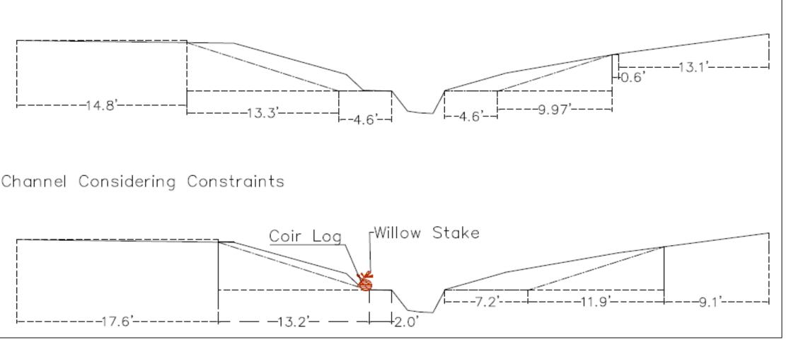
**Constructed 2-Stage Channel Cross Section Example**
